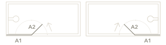
↔ DOOR OPENING DIRECTION ----- SWING RADIUS / PROTRUSION
